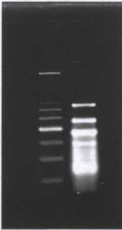
Figure 1: Banding pattern observed in one of the individuals in M. rosenbergii using RAMS primer, Bp11. Lane M: 100 bp marker, Lane 1: Bp11 primer bands
